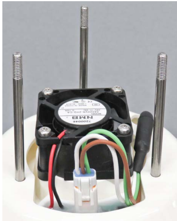
Figure 5: Cable routing after replacing the fan assembly
